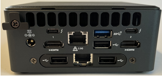
Figure 2: We tested transferring data through our data diode using an Intel NUC 11 Pro (NUC11TNHi50L). We used the bottom interface to send data to the top interface.
