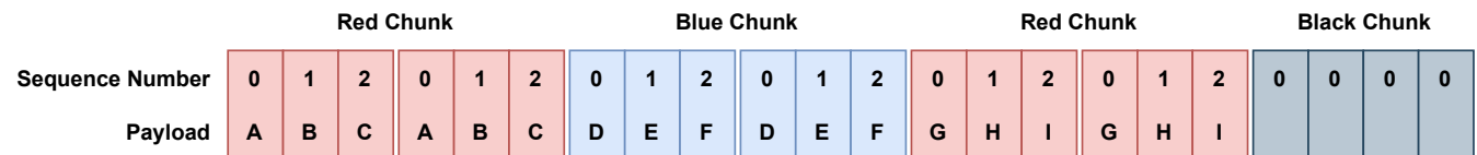
Figure 6: Our pydiode prototype sends packets in “chunks,” which alternate between “red” and “blue.” For resilience against packet loss, each chunk is transmitted a configurable number of times. The end-of-file is signalled by a “black” chunk. This diagram shows three distinct chunks of data, each of which is transmitted twice. Each chunk of data consists of three packets, with sequence numbers 0, 1, and 2. In practice, we sent data chunks with up to 100 packets each, which with a “redundancy” of two makes pydiode resilient to packet loss of up to 100 sequential packets.
